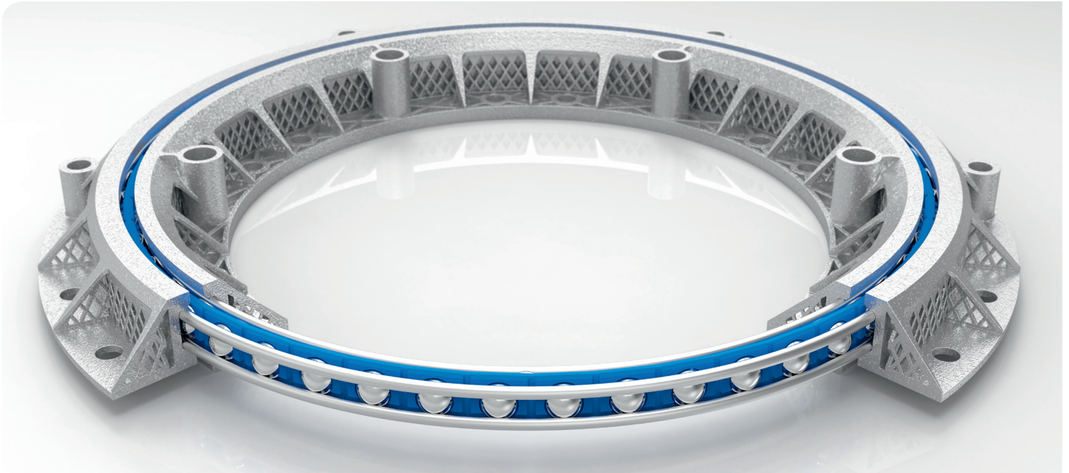
Franke lightweight bearing with housing made of 3D printing and integrated wire race bearing. Clearly visible is the filigree structure of the enclosing parts.
