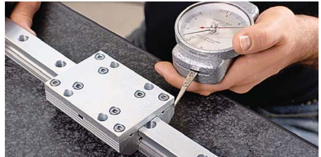
Diagram 2: Measure slide resistance (예압 측정)
