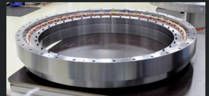
The special bearing assembly with integrated torque drive.
